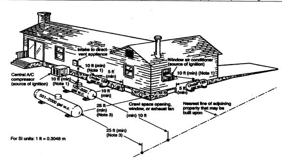
Note 1: Regardless of its size, any ASME container filled on site must be located so that the filling connection and fixed maximum liquid level gauge are at least 10 ft from any external source of ignition (e.g., open flame, window A/C, compressor), intake to direct-vented gas appliance, or intake to a mechanical ventilation system.
